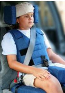
Adaptive boosters must be used with the vehicle's shoulder/lap belt system to provide restraint. The harness is for positioning only to provide supplemental support to a child with special health care needs. Depending on the booster, they may also have accessories that aid with positioning, such as abductor wedges, support pads, lap trays, foot props, and turning bases. Upper weight ranges vary from 80-175 pounds.
